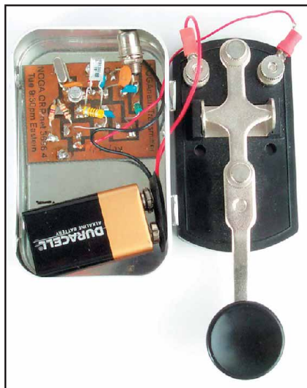
The NOGA naut 80-meter QRP transmitter, constructed by the author. This peanut whistle is described in the North Georgia QRP Club Compendium, Volume 1 .
