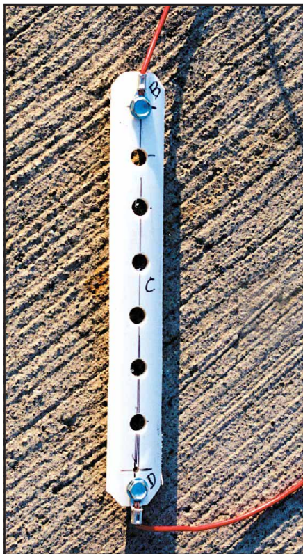
Figure 4—One of the two insulators for the wire elements.
